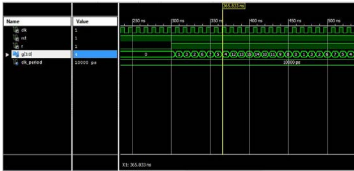
Fig9. Simulated waveform showing Gray counter output
